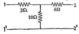
Q.7 a) Find the transmission parameter for the network shown.
