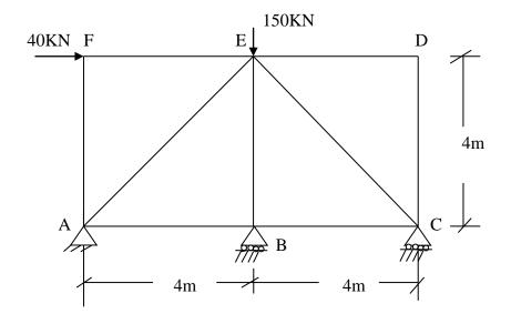
Q.5 Analyze the beam by using slope deflection method.
